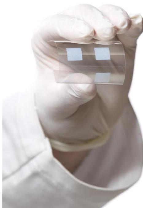
Figure 8. TiO<sub>2</sub>/SiO<sub>2</sub> hybrid nanocomposite flexible photoanodes inkjet-printed onto ITO/PET foil.
